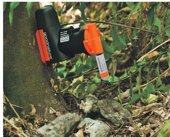
IMPRESSIVE: The self-resetting A24 traps registered 120 kills during the trial compared with just six for the single action Victor traps.
